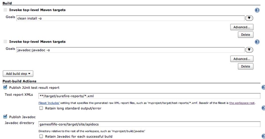
Figure 2.25. Adding a new build step and report to generate Javadoc
