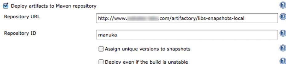
The screenshot shows the configuration for 'Deploy artifacts to Maven repository'. It includes a checked checkbox for the option, a text field for 'Repository URL' containing 'http://www. ....com/artifactory/libs-snapshots-local', a text field for 'Repository ID' containing 'manuka', and two unchecked checkboxes: 'Assign unique versions to snapshots' and 'Deploy even if the build is unstable'. Each field has a help icon to its right.
